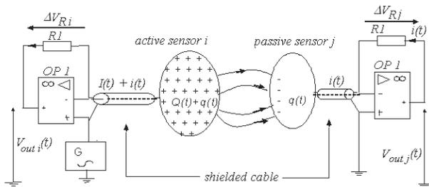
Fig. 20. Connection between the sensor and the linear integrated amplifier.
