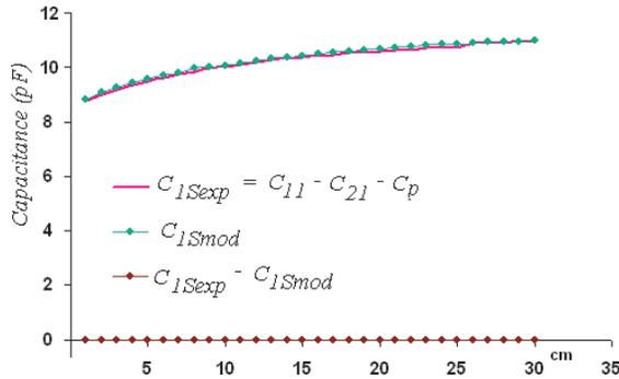
Fig. 9. Experimental model validation,  $\beta = 1$ ,  $C_{1Sexp}$  is the experimental capacitance curve,  $C_{1Smod}$  is the model, their difference is null,  $C_p$  is the capacitor of the shielded connection wire.
