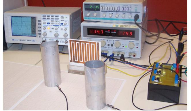
Fig. 7. Fabricated interdigital set-up and its associated electronic.
