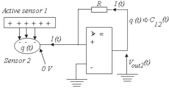
Fig. 5. Capacitive coupling and access to  $C_{12}$ .
