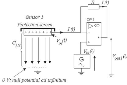
Fig. 4. Capacitive coupling and access to  $C_{11}$ .
