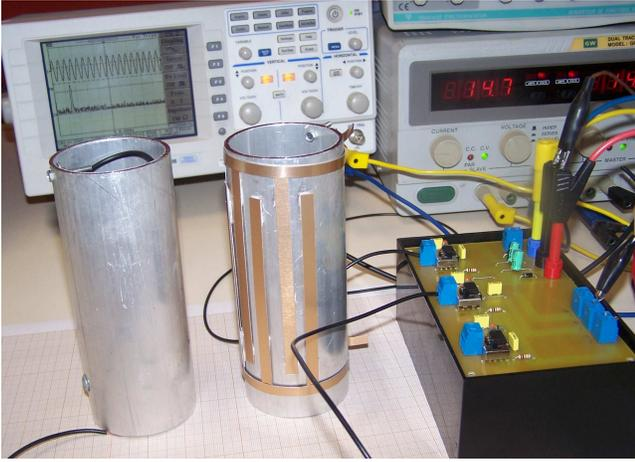
Fig. 8. Fabricated interdigital set-up and associated electronic.
