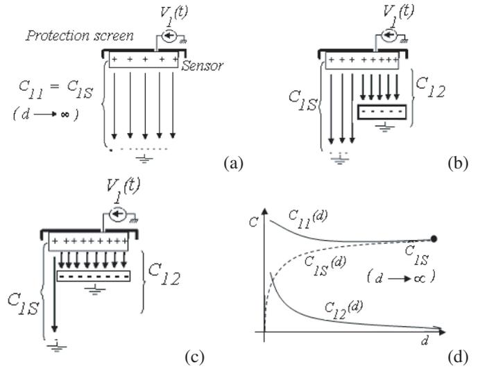
Fig. 2. Capacitance behavior of  $C_{11}$ ; a, b, c: Qualitative components of  $C_{11}$ , sensor-grounded target; d:  $C_{1s}$ ,  $C_{11}$  and  $C_{12}$  versus distance curves.
