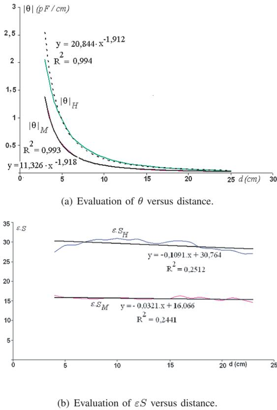
Fig. 17. Detection of an intrusion on the floor, index  $H$  for a man and  $M$  for a metallic target.
