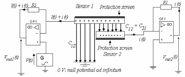
Fig. 6. Implementation scheme of the capacitive coupling translation.
