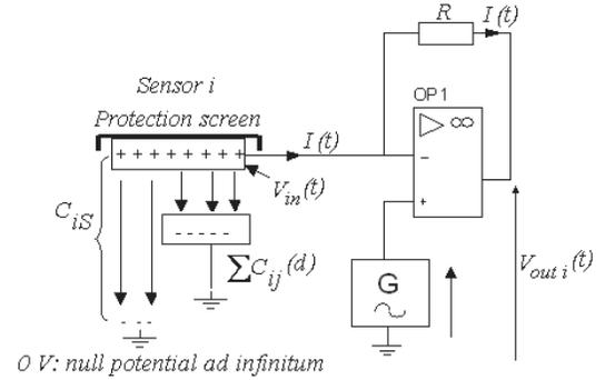
Fig. 10. Coupling translation for  $n - 1$  passive sensors.
