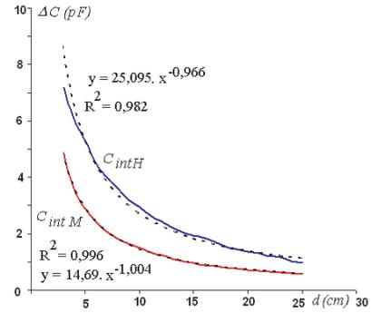
Fig. 16. Experimental results, coupling sensor-intruder versus distance :  $C_{intH}$  for a human,  $C_{intM}$  for a metallic target.
