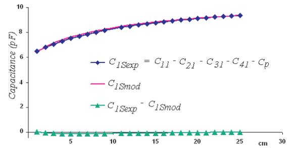
Fig. 11. Experimental model validation,  $\beta = 0.2$ ,  $C_{1Sexp}$  is the experimental capacitance curve,  $C_{1Smod}$  is the model, their difference is null.
