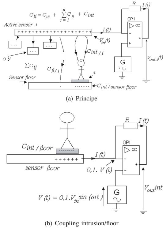
Fig. 14. Detection of an intrusion on the floor.
